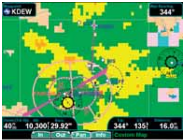
Graphical NEXRAD via XM Satellite Radio and GDL 69
