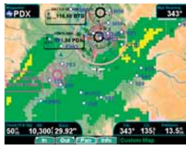
Custom map feature allows the pilot to overlay some or all of the GMX 200 features.
