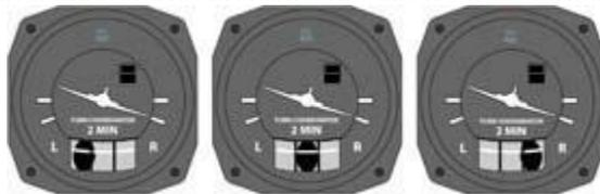
The inclinometer or "coordinator ball" shows the relationship between the bank angle and the rate of yaw. The turn is "coordinated" when the ball is centered. The aircraft is "skidding" when the ball rolls toward the outside of the turn and is "slipping" when it moves toward the inside.
